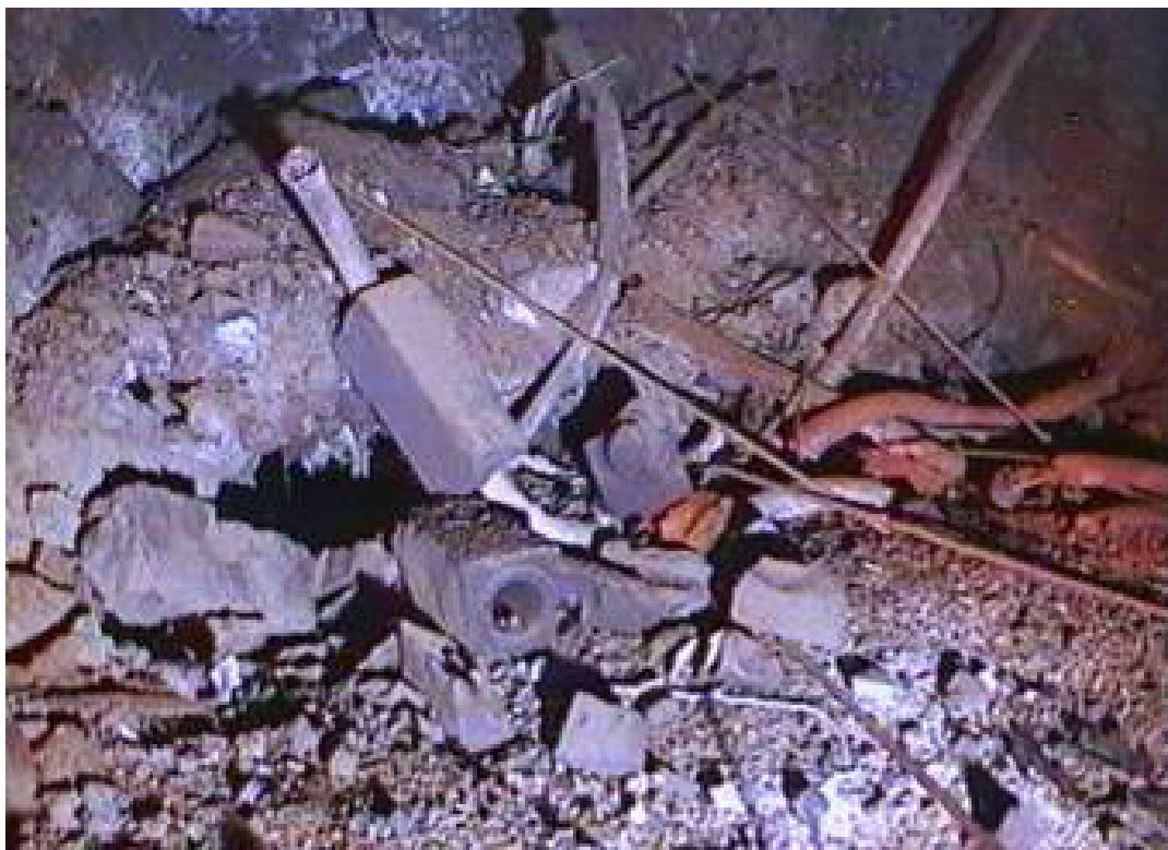
Fig. 5.1. Fragments of destroyed reactor core in premise 305/2.
